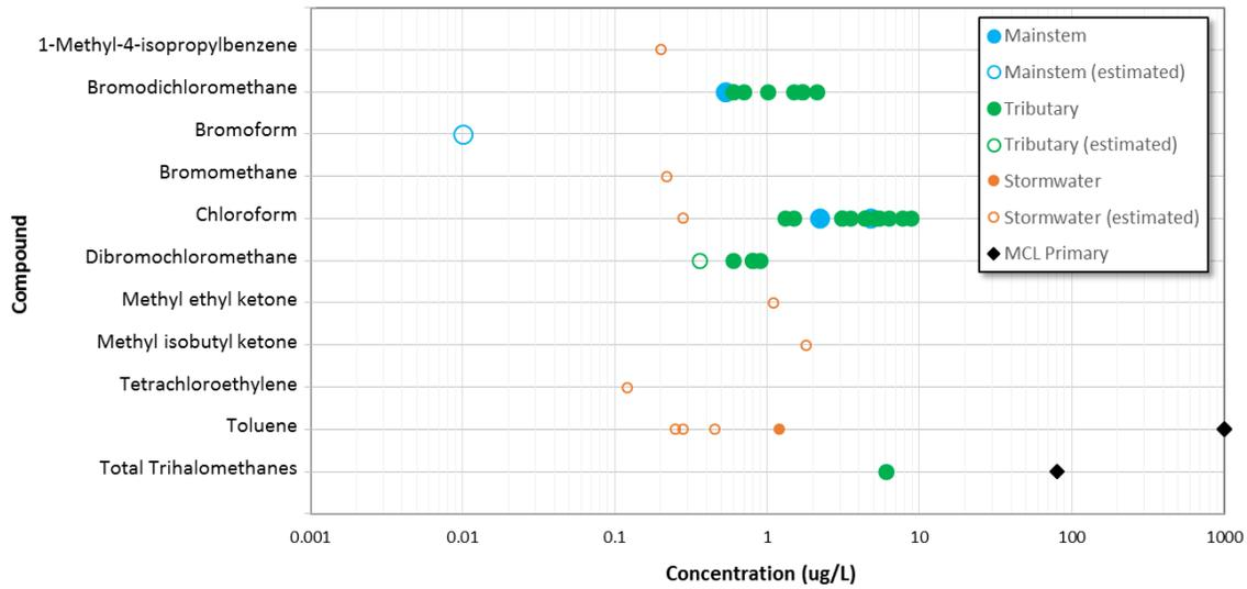
**Figure 5-22: SVOC Detections in the McKenzie Watershed by Channel Type, 2000-2016**
