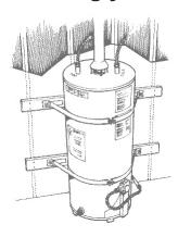
Water heaters can move or tip over if not securely anchored to the wall or floor. For a small investment of time and money, you can avoid spilling gallons of precious water that could be useful in an emergency.
