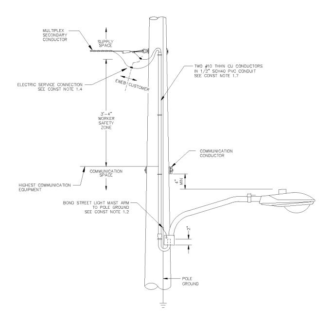
REQUIREMENTS FOR STREETLIGHTS MOUNTED IN THE COMMUNICATION SPACE
