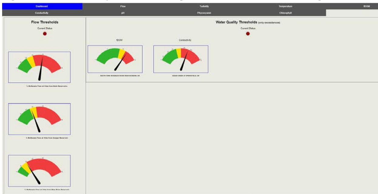
Figure 1-2: Water Quality Dashboard using Data from Real-time Monitoring Stations
