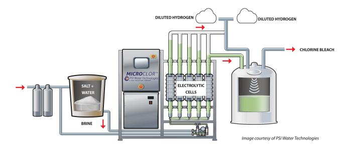
SALT + WATER + ELECTRICITY = CHLORINE BLEACH (SODIUM HYPOCHLORITE) + HYDROGEN GAS NACI + H2O + ELECTRICITY = NAOCL + H2
