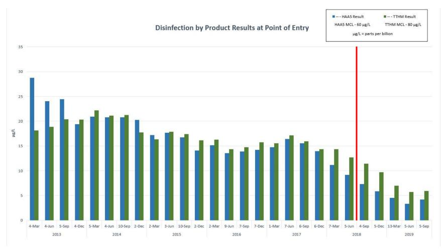
**Note:** The red line indicates when biofiltration was added to the treatment process which further reduced organic material in the water.
