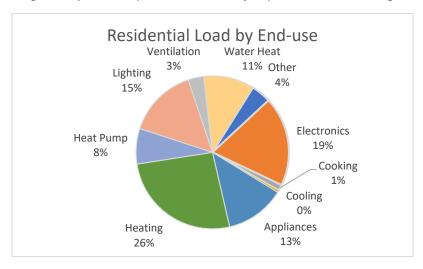
Figure Y– Space heating accounts for about 34% of EWEB's total residential load, while water heating adds another 11%<sup>28</sup>.
