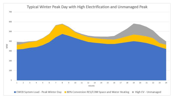
Figure TT- Electrification of space and water heating accentuates the morning peak, while the additional load associated with EV charging creates a second evening peak.
