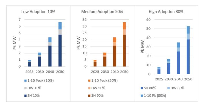
Figure II— Peak impacts to the utility are dependent on the amount of commercial space and water heating electrification which occurs over time but are also increased by colder than average weather (1-in-10).
