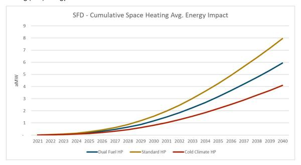
The peak impacts of these technology choices are significant, as cold climate heat pumps are able to utilize the compressor at very low temperatures and reduce reliance on backup electric heat. Dual fuel heat pumps are assumed to switch over to natural gas below 32 degrees Fahrenheit, meaning they would add only a minimal amount to EWEB's existing peak load. For context, EWEB's existing 1-in-10 peak system load is 510 MW.
