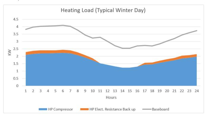
Figure R – Modeled energy use of a heat pump (HP) system compared to baseboard heating.
