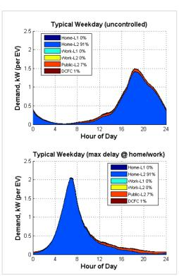
Figure N – Comparison of uncontrolled and controlled EV charging behavior shows that the timing and load shape of energy consumption can be changed.
