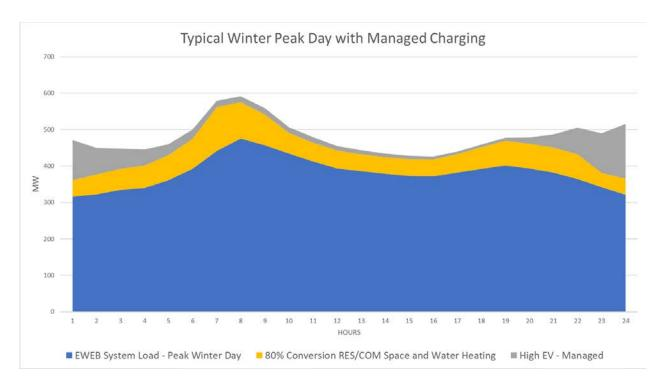
Figure UU- Shifting peak EV charging from 7 PM to 12AM (off-peak) moves the EV charging load away from EWEB's system peak and results in lower energy costs and much lower carbon emissions.
