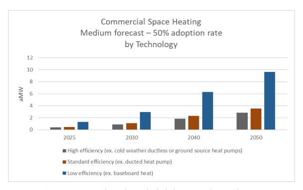
Figure FF – Commercial space heating load is higher compared to water heating, and the efficiency of electrified heating equipment is important.
