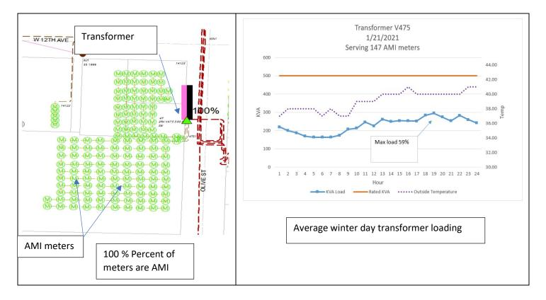
Each connected meter (child) is assigned to its virtual transformer (parent). Hourly load data from each of the individual meters is summed for each hour and the maximum hourly load can be compared to the transformer's capacity rating, as illustrated in the image on the right.
