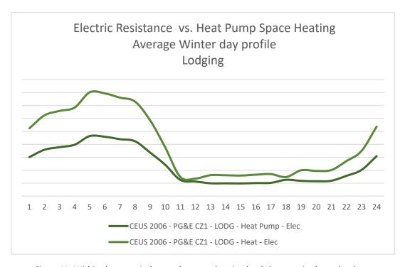
Figure V - Within the same industry, the space heating load shape varies by technology.
