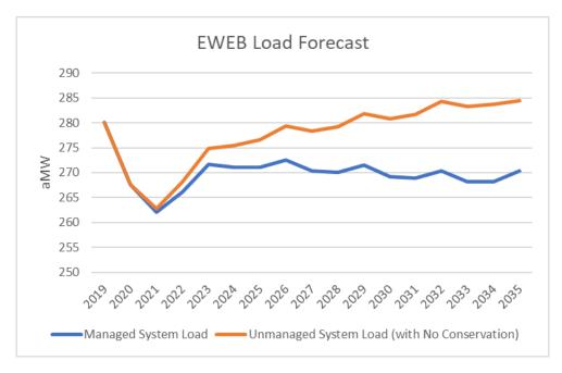
Figure B - Average load forecasts show little to no load growth (Managed System Load is net of conservation)
