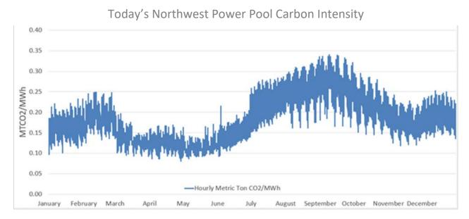
Figure A - The hourly carbon emission for the NWPP region based on Aurora modeling software. The areas used by EWEB for modeling the NWPP region may differ from the actual physical boundaries of the NWPP but is intended to illustrate the region's carbon intensity.
