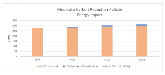
Figure NN – Absent aggressive carbon reduction policy, conversion of space and water heating end-uses is expected to remain sluggish and the average energy impacts lessen to an increase of 7%.
