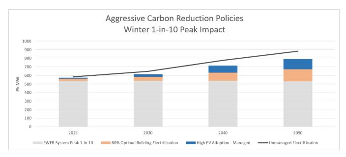
Figure OO - High levels of electrification could add between 49-66% to EWEB's existing 1-in-10 peak
