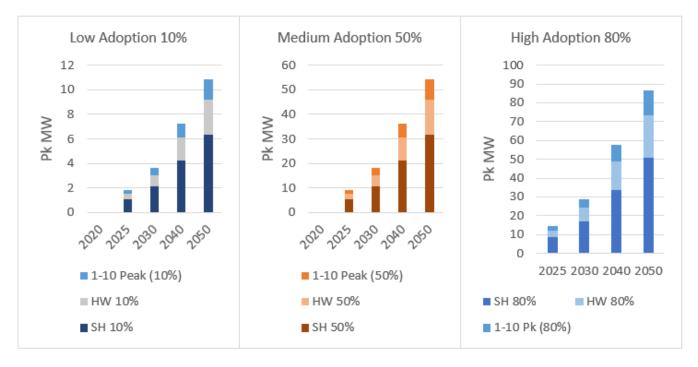
Figure CC—Peak impacts to the utility are dependent on the amount of space and water heating electrification which occurs over time but are also increased by colder than average weather (1-in-10).
