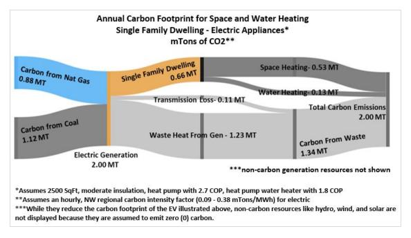
Figure KK – The majority of energy from electricity is carbon-free. However, electricity generated with natural gas and coal must be considered in the carbon footprint.
