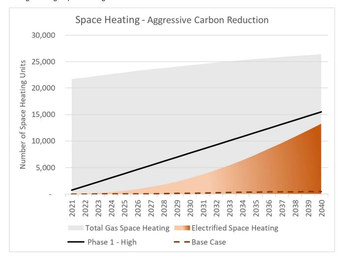
For space heating electrification, the choice of technology has a strong influence over the average and peak energy impacts to the utility. To illustrate the impacts, the charts below show the energy impacts assuming 100% of the units electrified chose the same space heating technology. The results are shown based on single family dwelling (SFD) energy use.
