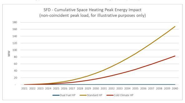
The chart above shows the non-coincident peak load of electrifying space heating units. The coincident peak impacts are anticipated to be much lower, as equipment diversity and customer behavior reduce the system peak impacts the utility would see as a result of electrification. It should also be noted that different customers will choose different space heating technologies, so the impacts are further diversified by different equipment types.
